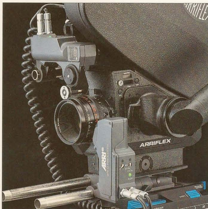
Focus- and iris-control on the ARRIFFLEX 35 III with a short-sized lens and an iris ring that varies with the distance adjusted
